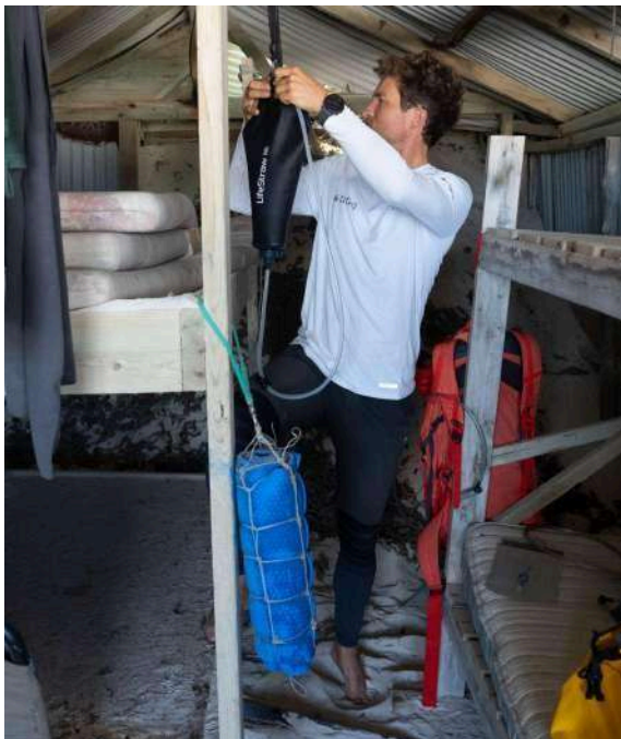
Rainwater filtration using a LifeStraw Gravity system
