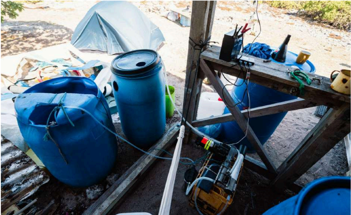
Solar-powered watermaker producing freshwater at DJL camp
