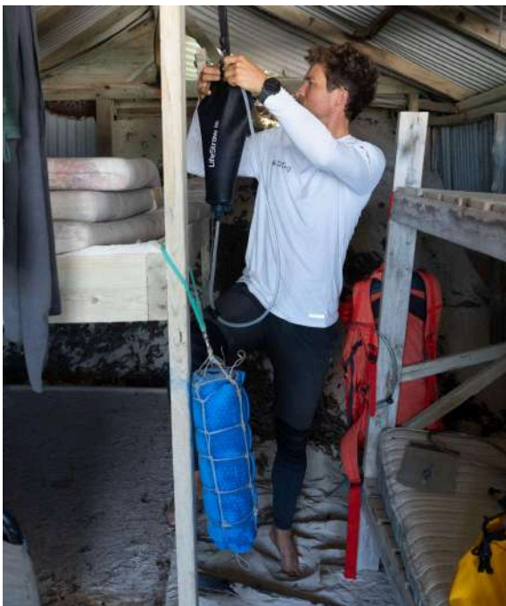
Rainwater filtration using a LifeStraw Gravity system
