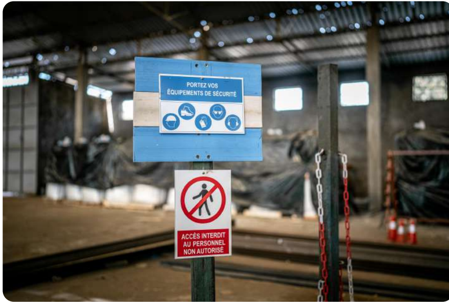
FIG-10 Basic PPE required for every POF factory: hearing, respiratory, eye, hand protection.
