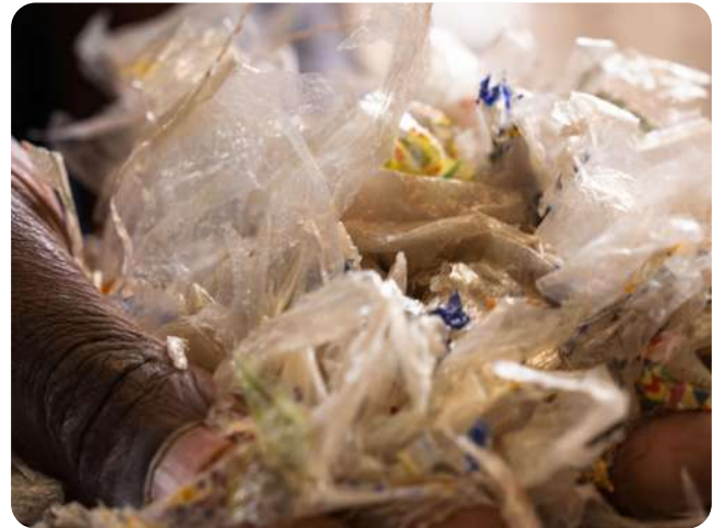
FIG-08 – Handful of shredded LDPE film flakes, Dakar collection.
