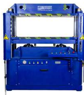
(e) Hydraulic press with moulds
