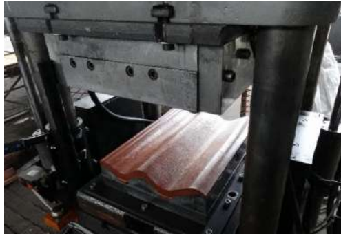
Roof tiles in the press with its mold above
