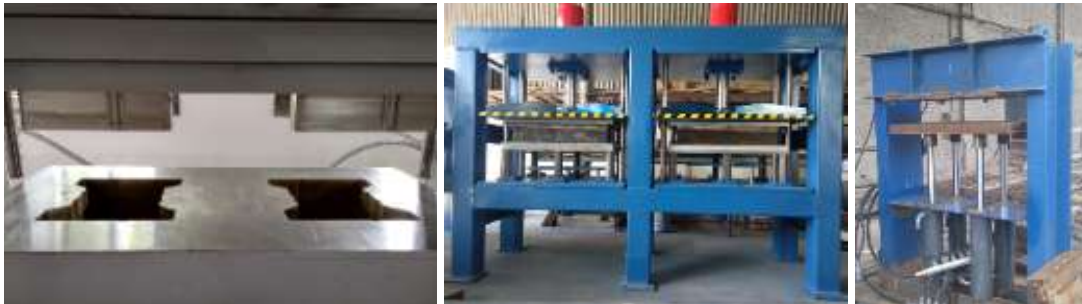
More efficient hydraulic press (2 pavers at a time) - Double or single hydraulic press
