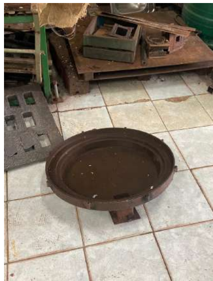
Mould for manhole cover with integrated sign
